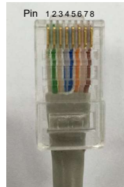
RJ45 Terminal Configuration of Meter/CT Communication
