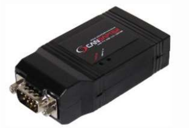
Figure 2.3 CANdapter for Programming Freedom Lite Business 80/56 model
